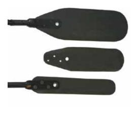
A MaxCell Rodder Head or "paddle" is the most effective tool for overriding existing cable plant. Insertion of the paddle over the top of existing cables presses the cables down in the conduit, creating a larger open space at the top for the placement of MaxCell and subsequent additional cable. The correct size of the Rodder Head selected for any application depends on several factors, including:
